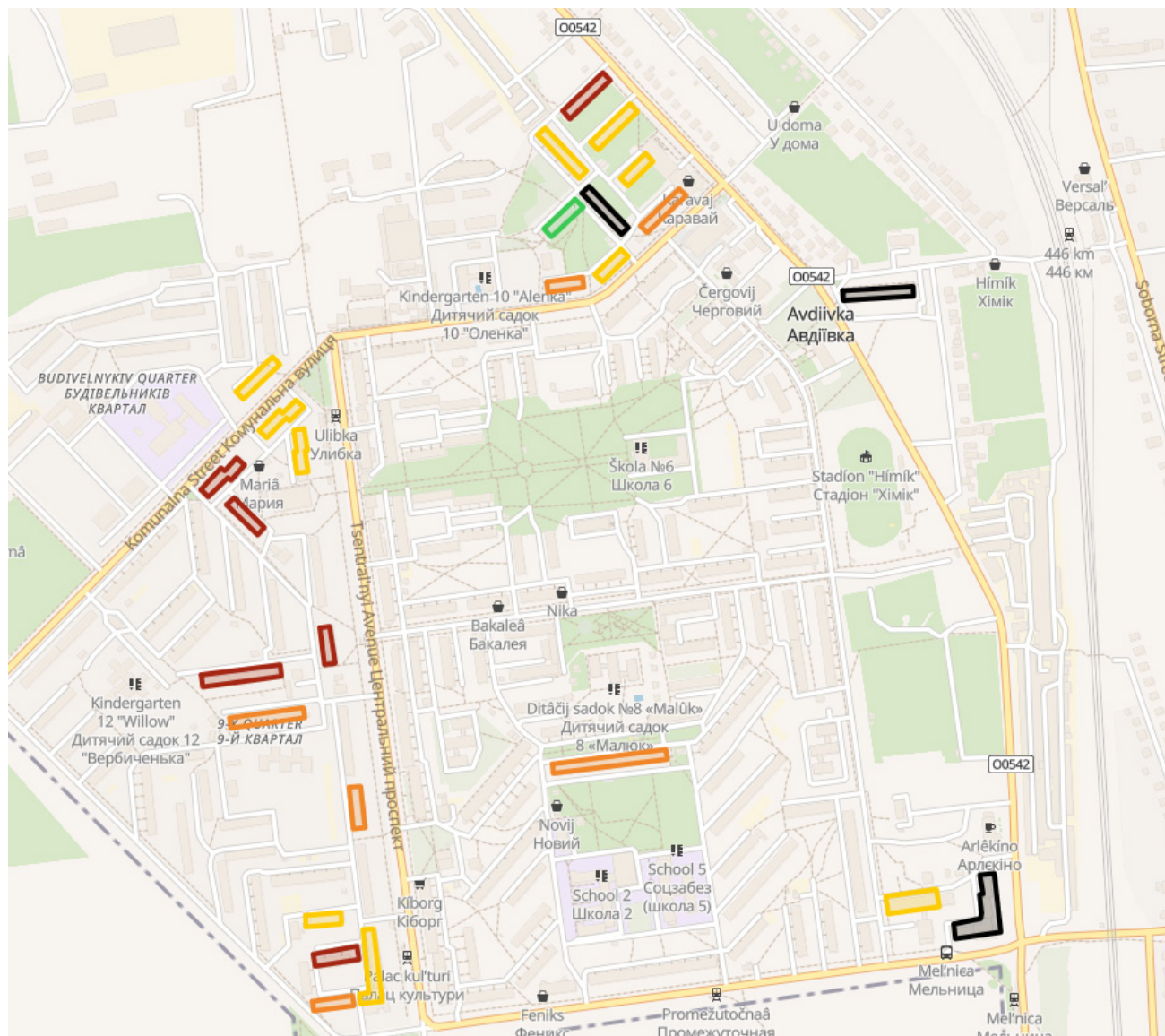
Figure 5: Overview of damage to Avdiivka's 26 high-rise buildings between February 2022 and 21 November 2023. Destroyed buildings are marked in black (three) , partially destroyed in red (six) , moderately damaged (including fire damage) in orange (four) , lightly damaged in yellow (ten) , and buildings with no damage reported in green (one) .
