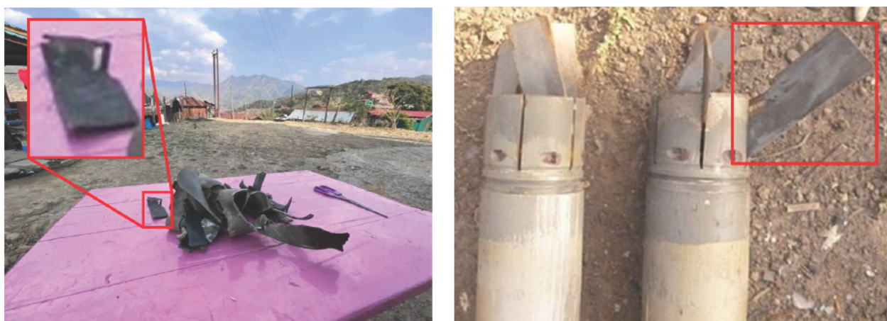
Figure 10: Visual comparison of remnants from Khuafu (left) to confirmed S-8-type rockets' fins sections (right) (sources: The Chin Journal ; Myanmar Witness ).
