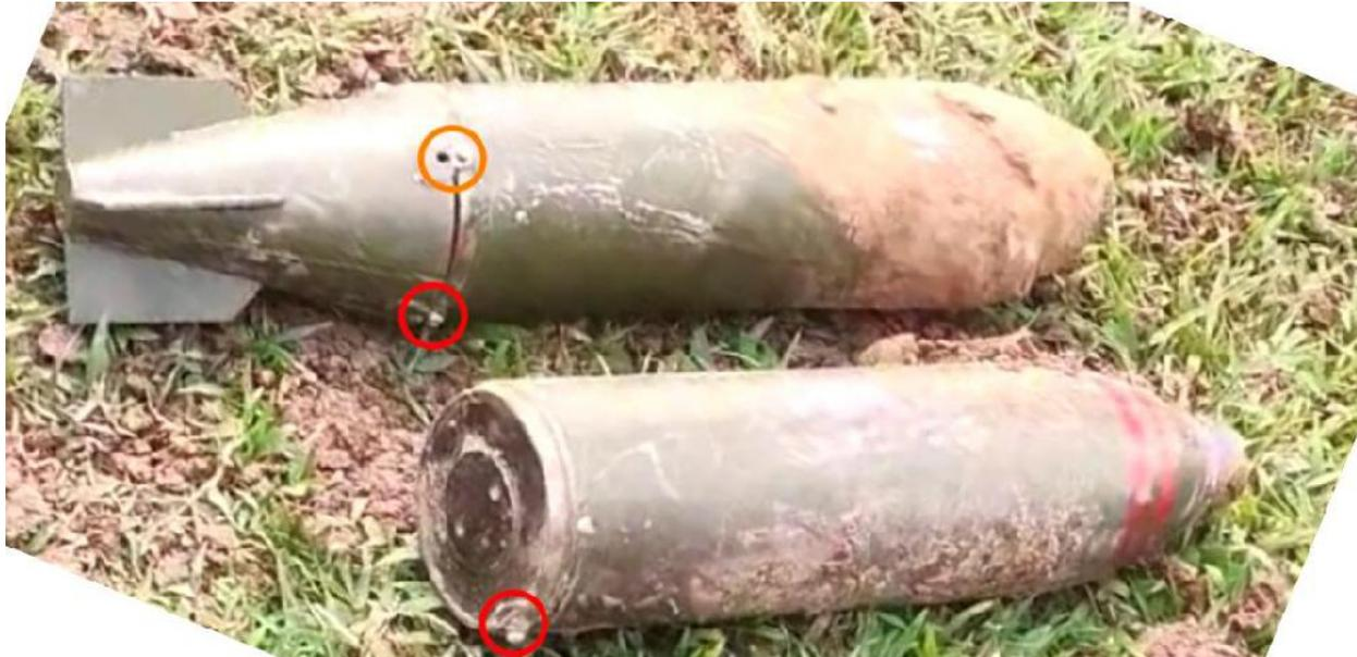
*Figure 19: The presence of screws on the first munition from the bottom suggests that a tail kit may have been initially attached. (Source: Private)*
