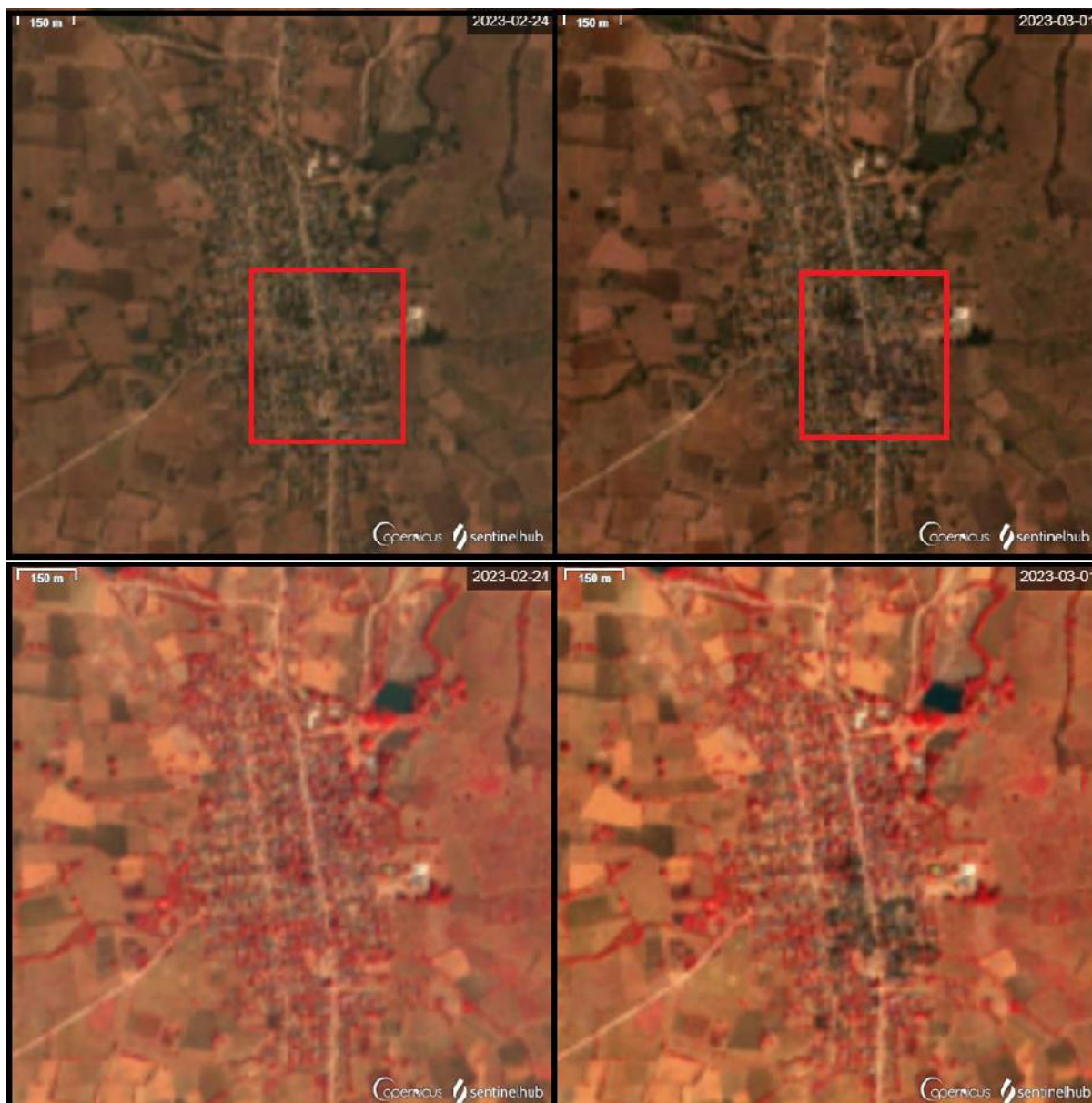
Figure 6: Sentinel data showing fire damage in Pa Dat Taing from 24 February to 1 March 2023. Top image shows visible light changes - showing the appearance of a slightly darker tone to the region affected. The bottom imagery shows Fire damage using false colour scales to emphasise vegetation alterations. Both show a high level of physical damage to the area.
