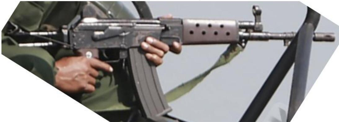
Figure 28: [Military Today](#) website shows a right-side view of an MA-3 Mk. II assault rifle. Notice the skeletonized side-folding stock and the short gas block which are a match with images 42-44 above and distinctive features of this model.
